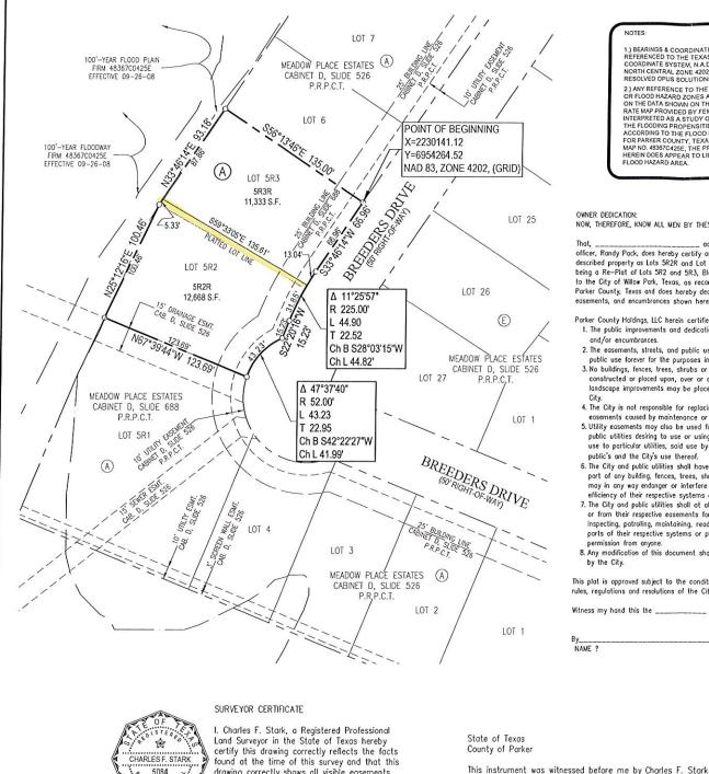
1.) BEARINGS & COORDINATES SHOWN HEREON ARE REFERENCED TO THE TEXAS STATE PLANE COORDINATE SYSTEM, N. A.D. 83 DATUM (TEXAS NORTH CENTRAL ZONE 4202) DERIVED FROM RESOLVED OPUS SOLUTIONS.
